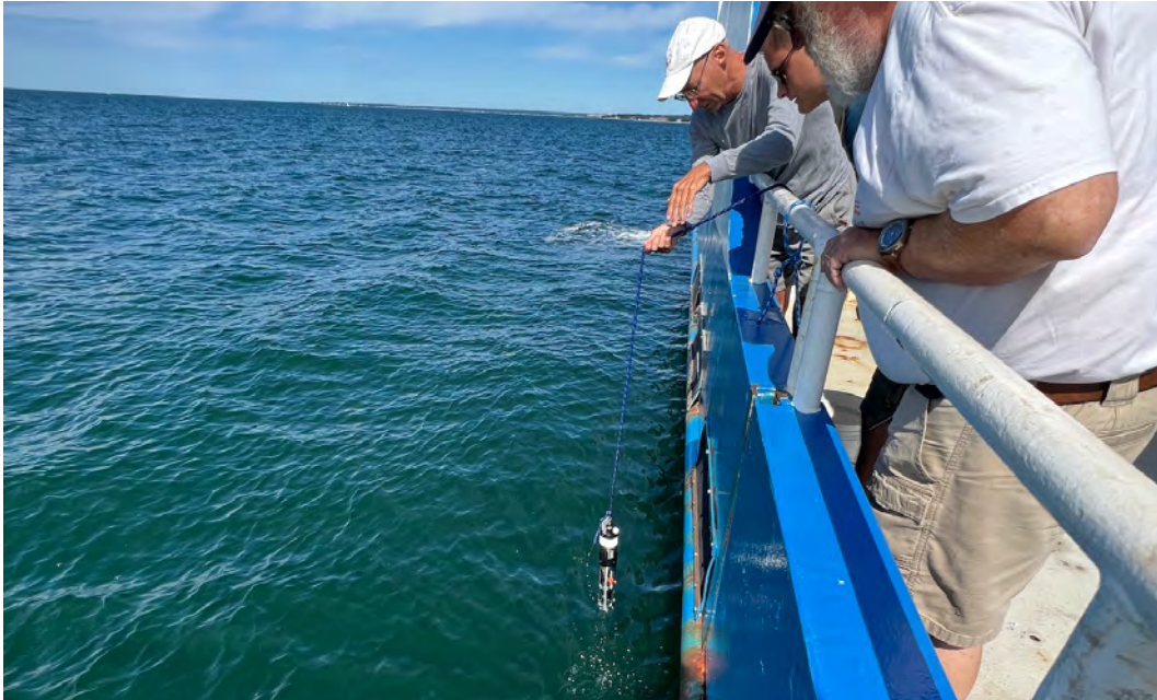
Figure 2-6 Dennis Arbige recovering the CTD used for sound velocity profile measurements.
