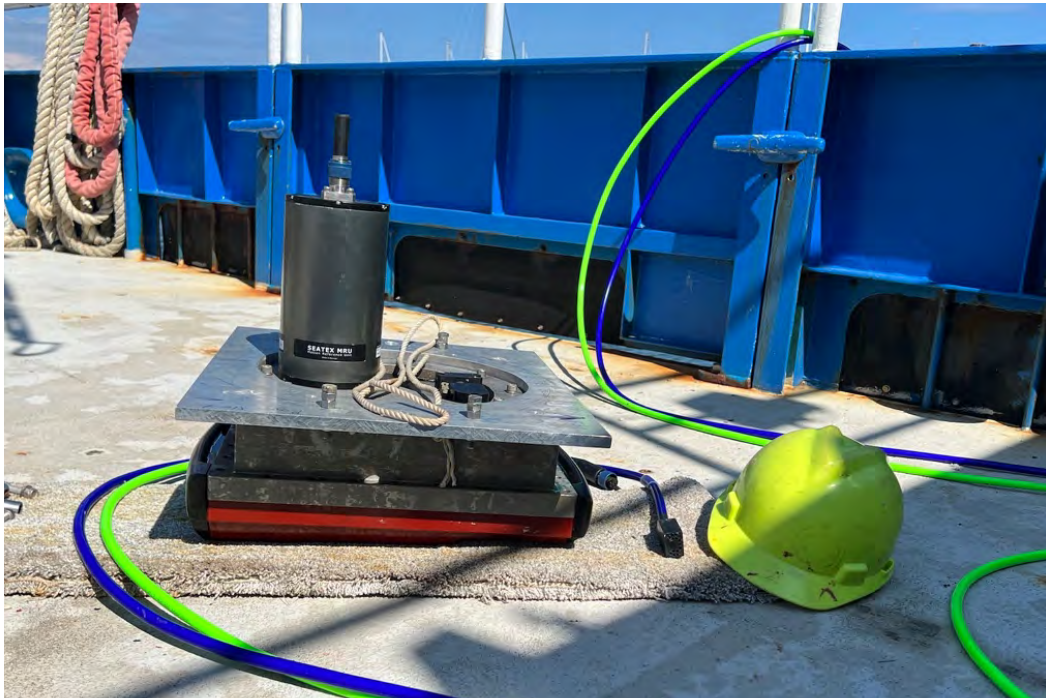
Figure 2-1 The acoustic transducer (bottom), mounting plate and motion reference unit (cylinder on top of plate) on the deck of the RV Connecticut.
