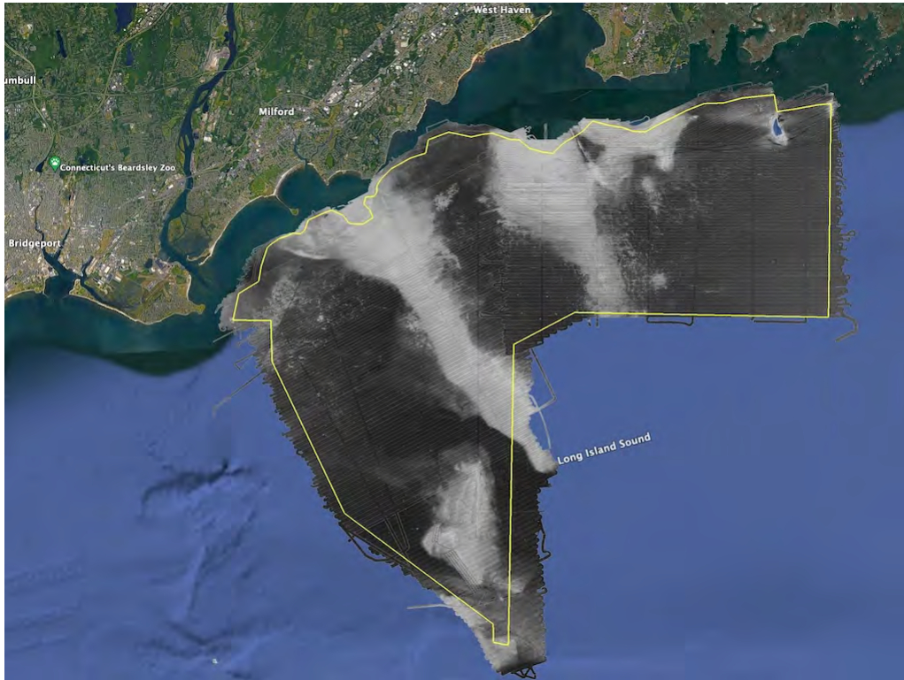
Figure 2-9 1 Compiled preliminary backscatter of the newly acquired acoustic data for the Phase IV area (outlined in yellow).
