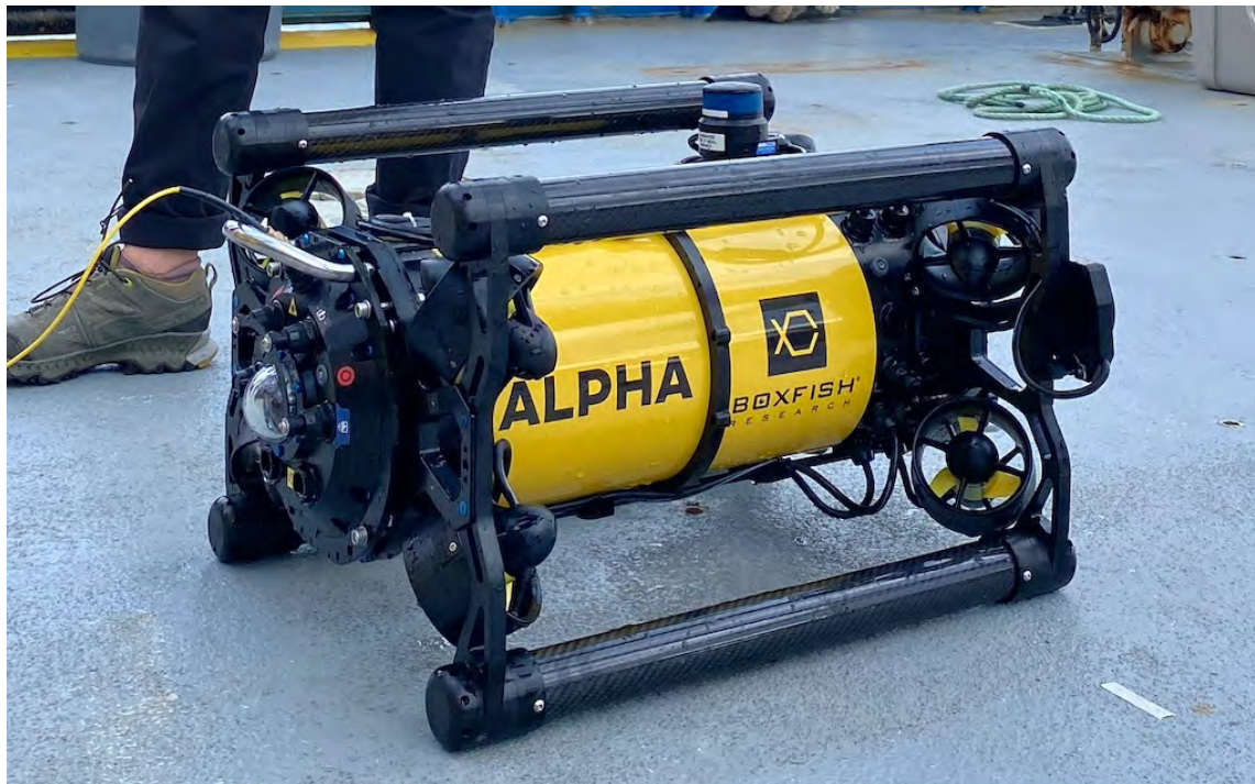
Figure 4-6 The Boxfish Alpha ROV on the deck of the RV Connecticut. Note the thin fiber optic tether (yellow) that provides control to and 4K video from the ROV.
